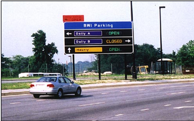
Figure 38: Example of Intelligent Signage
